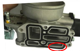
Seal leakage affects intake air flow
